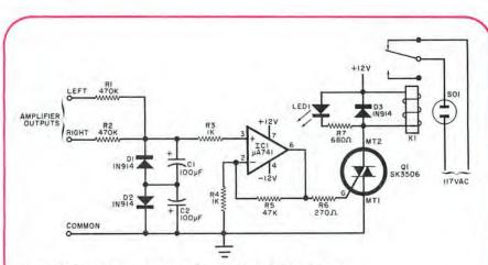
An unbalance across capacitors C1 and C2 triggers Q1 and energizes K1 to shut off the amplifier power.
