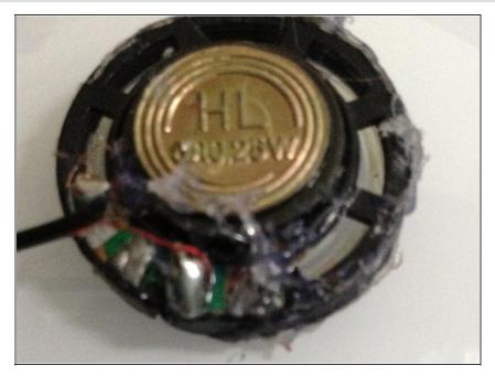
Cut about 10cm off of the audio cable, then strip the wire as in the picture. For wires that are coated with enamel, use a file to scrape the enamel off. Solder the wires to the solder tabs on the speaker.
