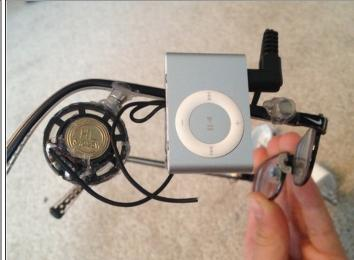
Plug the audio cable into the MP3 player's stereo jack. Then clip the MP3 player onto the glasses and attach the speaker to the glasses.
