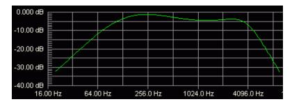
Similar cabinet simulators are utilized in Marshall amps - they have an additional frequency boost close to speaker's resonant frequency.
