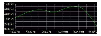
MP2 preamp by ADA has a possibility to to switch on or off additional Notch filters. The schematic available in the Internet can be hardly read, but our colleague RRysiek managed to draw the cabsim part. His schematic and modifications suggested by him can be found <a href="here">here</a>. Below there is a frequency response:
