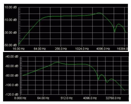
However, speaker cabinet's frequency response does not consist only of high and low frequency reduction and speaker's resonant frequency boost. In between we will find lots of "peaks" and "notches", which are results of many factors like: speaker type, speaker enclosure mechanics, or - very importantly - the cabinet surrounding. The actual frequency
