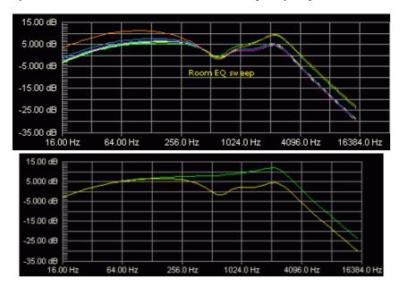
Another quite interesting circuit that provides vast modification possibilities is the **Varicab** module used in **ADA** amps. Electronically (schematic) it's a set of gyrators + two additional low and high pass filters. According to the manufacturer, the circuit offers simulation of all the common guitar cabinet types: 1x12", 2x12", 2x10", 4x12". Let's take a look at the frequency response diagrams:
