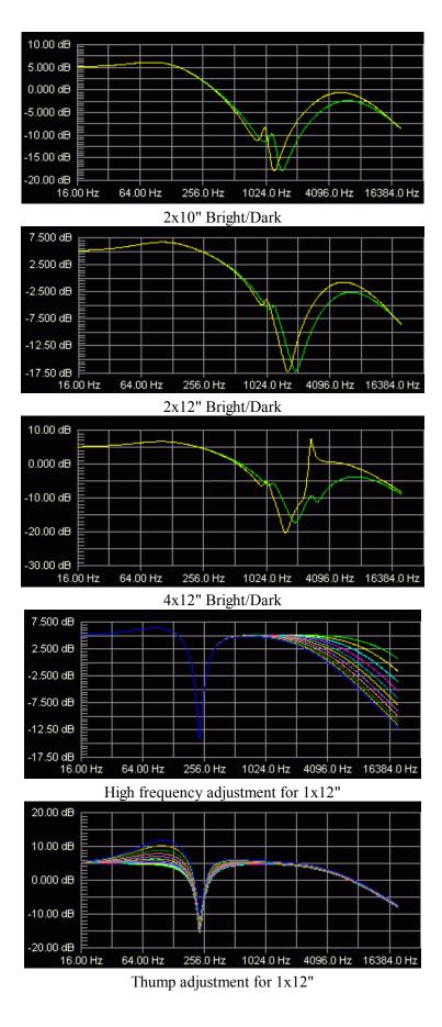
And finally two "cherries on the cake" - the most complex circuits that most accurately simulate the speaker enclosure's frequency response. These are devices designed by guys from <u>LHX2</u> Web site. Please visit their Web site for details. The circuits simulate the sounds of two main brands: Fender and Marshall. Shown are the frequency responses of these
