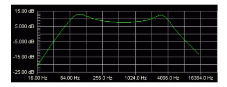
The next preamp by Mesa Boogie - **V-Twin** - has a simple filter, which can deliver purring blues tones. As usual for Mesa, the filter is based on inductance. Its <u>schematic</u>, <u>sound sample</u>, and frequency response:
