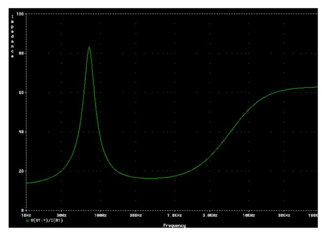
These circuits are designed to present a 16 ohm nominal load to the amp; if you want a different impedance, you will have to scale the resistive and reactive elements accordingly. The impedance scaling factor will be Z = Znew / Zold, and the new element values will be as follows:
