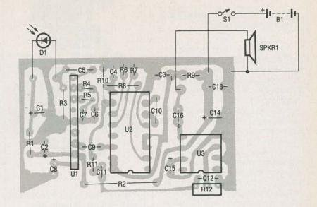
Fig. 6. The receiver's printed-circuit board should be assembled using <sup>1</sup>/<sub>8</sub>-watt or smaller resistors and miniature (radial lead electrolytic and ceramic-disc) capacitors. The volume control (R12) can be a miniature PC-mounted potentiometer or conventional unit, which would have to be mounted off-board.
