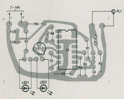
Fig. 5. The size of the parts used to build the transmitter are important due to space constraints, thus, <sup>1</sup>/<sub>4</sub>-watt or smaller resistors are a must and miniature (radial lead electrolytic or otherwise) capacitors are recommended.
