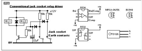
Figure 2 - Alternative Relay Driver, and Component Pinouts
