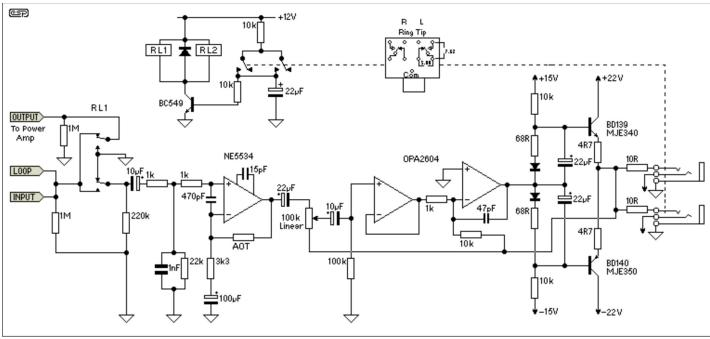
Figure 1 - The Headphone Amp Circuit
