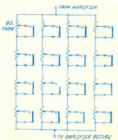
faders in series. The net impedance of the circuit is eight ohms, an ideal load for your Fisher. One nice feature of this simple circuit
