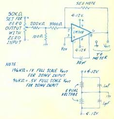
amps have an offset null input, but the LM308 does not. But it does have the high
