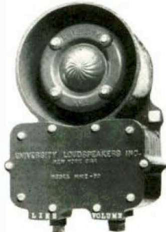
Fig. 6. Speech type horn loudspeaker designed for railroads, mines and hazardous locations. It has a throat diameter of 2 1/2 inches, an air column length of only 8 inches, is characterized by wide dispersion angle.
