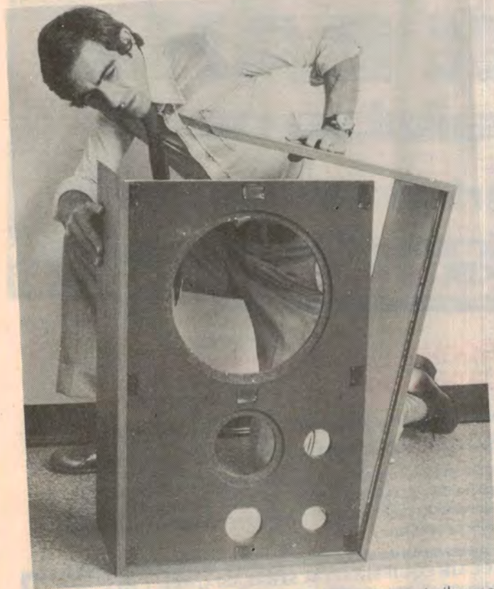
Assistant Editor Greg Swain shows how a typical pre-cut cabinet kit goes together, with the top of enclosure on the floor. In this way, the corner joint will normally be out of sight.
