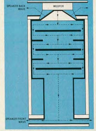
FIG. 1—SAFE EFFECT uses both the front and back waves from the woofer to extend bass response. The front wave travels through an acoustically long labyrinth to increase apparent size of enclosure.
