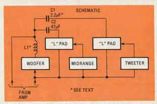
FIG. 4—SIX dB/OCTAVE crossover network is simple to build. L-pads balance sound from the three sections of the system.
