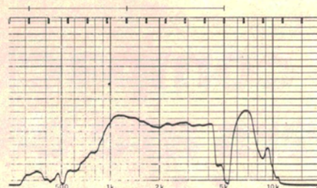
Mid-range. Its piston operating range extends from about 1 kHz to about 4.5 kHz.
