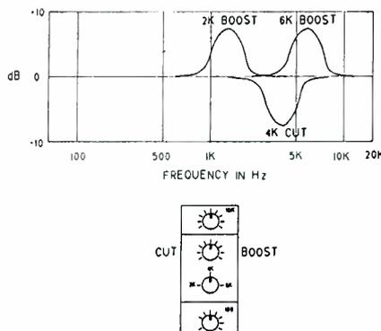
When the controls are adjusted, their positions graphically indicate the resulting frequency response. Usually, a graphic equalizer is used for monitor-speaker EQ.
