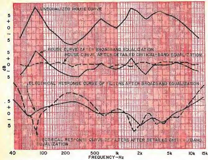
Fig. 3. Attempts to equalize a playback channel with broadband ( $\frac{1}{3}$ -octave) filters compared to critical-band ( $\frac{1}{3}$ -octave) filters.
