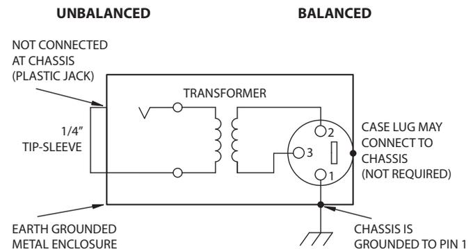
Figure 2. Transformer Isolation
