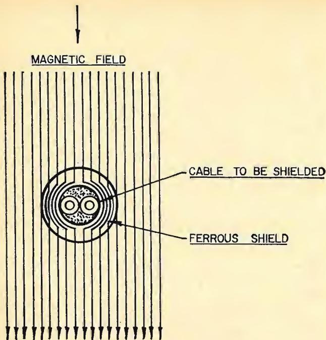
Fig. 4. Ferrous materials repel external lines of flux.
