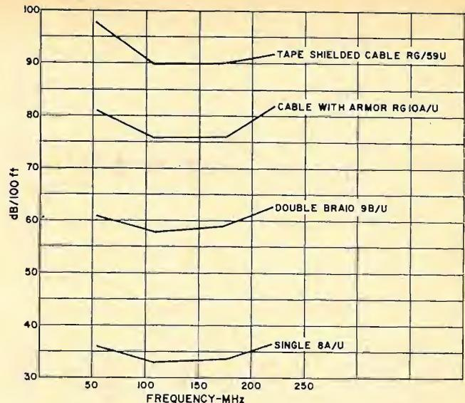
Fig. 3 Relative shielding efficiencies for various cables.
