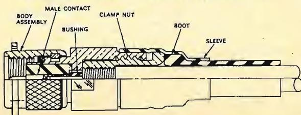
Braided cables cannot be used at the higher radio frequencies—above 6 GHz—because of high signal loss through the braid. And when the braid is flexed, the attenuation varies widely, indicating unstable shielding effectiveness. A flexed braid is also a noise source.
