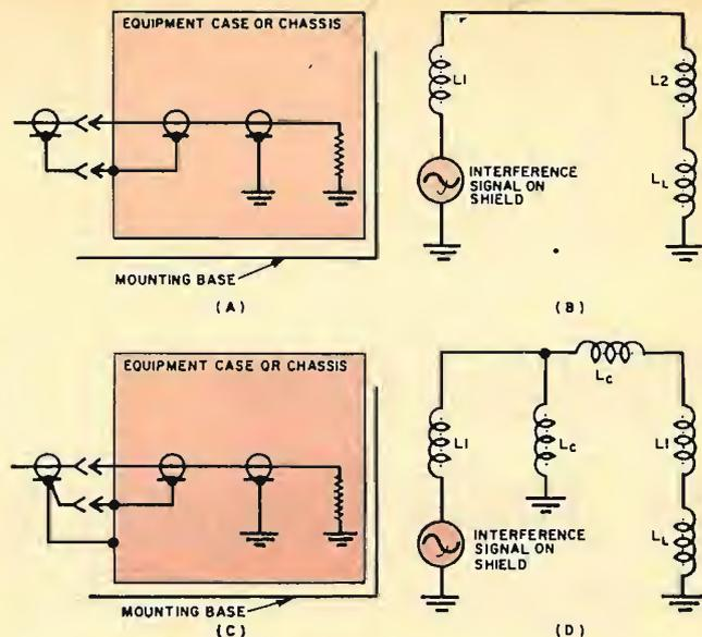
Fig. 5. Poor bonds permit noise to enter equipment.
