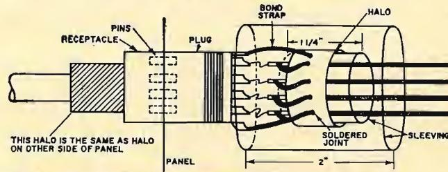
NOTES: 1. BOND STRAP MAY BE CONNECTED AS SHOWN OR WITH 1/4" BOND STRAP TIED TO STRUCTURE OR CONNECTED BY MEANS OF EARED WASHER
