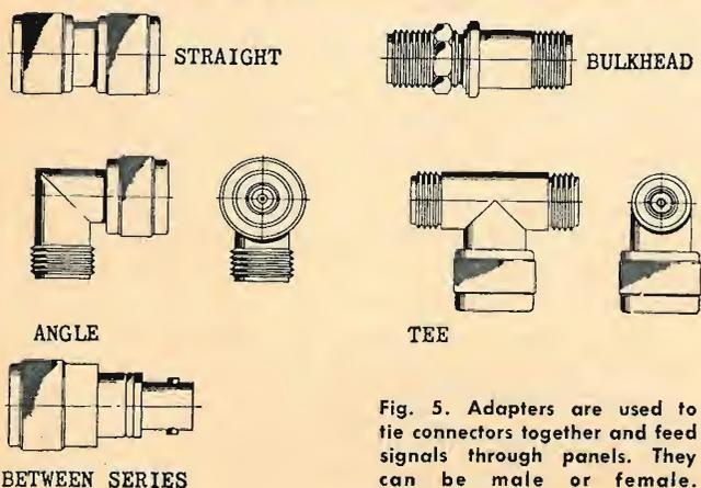
Fig. 5. Adapters are used to tie connectors together and feed signals through panels. They can be male or female.
