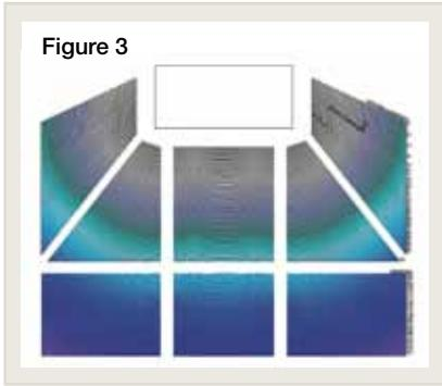
VARIA's flexibility in coverage patterns enabled a design where all arrays can line up precisely to each major seating section, creating strong acoustical cues to the stage (Figure 3). The arrays were designed strictly around angular coverage requirements.
