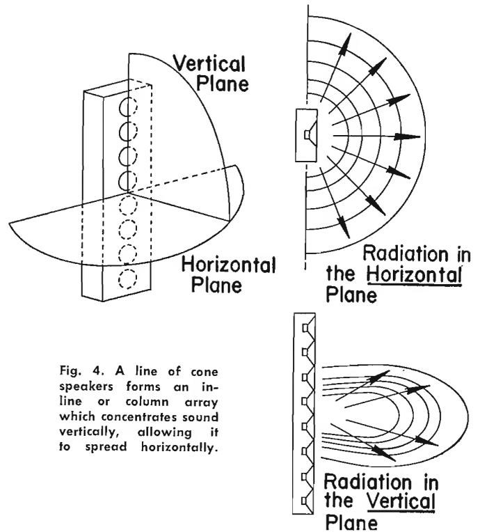
Fig. 4. A line of cone speakers forms an in-line or column array which concentrates sound vertically, allowing it to spread horizontally.
