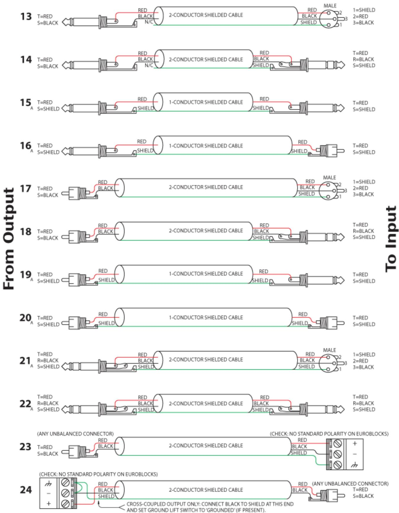
Figure 4. Interconnect chart for locating correct cable assemblies.
