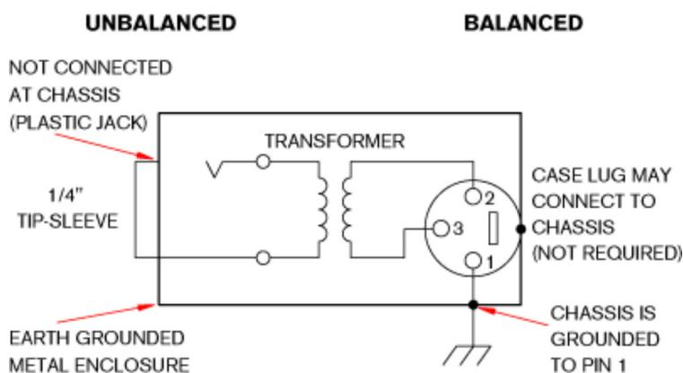
Figure 2. Transformer Isolation
