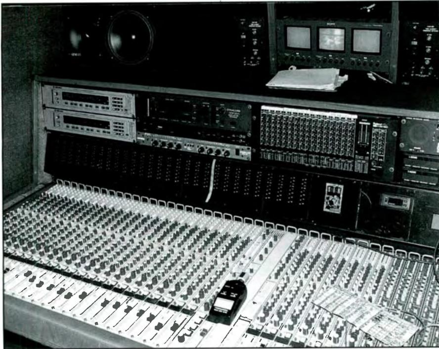
Figure 4. The dominant feature at the front of the room is the 36 channel Harrison MR-4 console.
