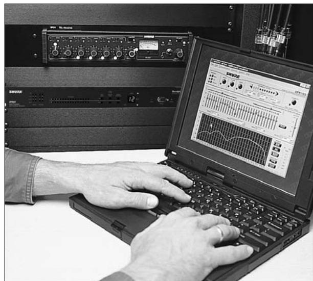
Example of a PC-controlled Feedback Reducer and Equalizer.
