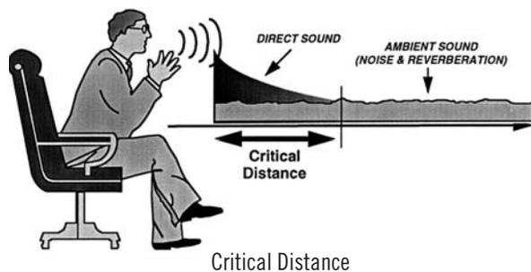
This brings up the concept of “reach”, or distant pickup capability. The proportion of direct vs. ambient sound picked up by a microphone is a function not only of distance but of the directional pattern of the microphone as well. For a given ratio of direct-to-ambient sound, a
