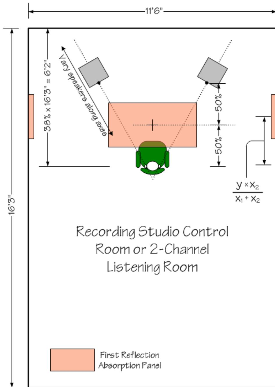
**Figure 1:** Proposed layout and first reflection points for a 2-Channel listening room.
