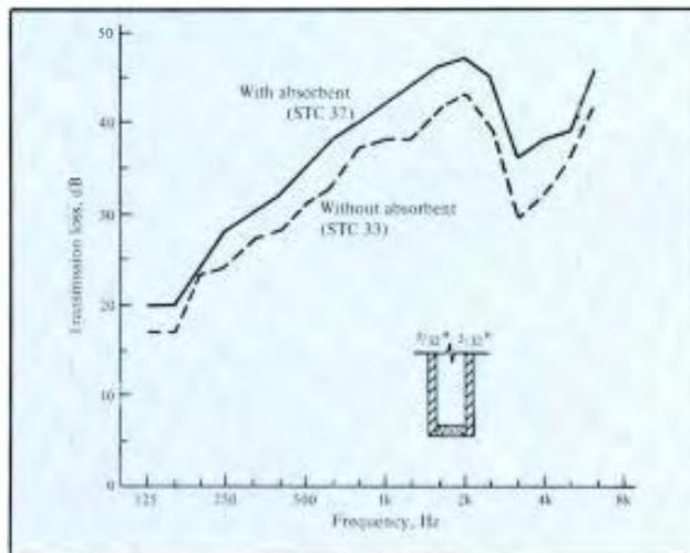
Figure 1. Actual measurements showing improvement of transmission loss of double glazed windows by covering the edges of the interpane cavity with sound absorbing material. A gain of 4 STC points is attributable to the absorbent. In this case, 5/32-inch (4mm) glass is used. Improvement of TL due to absorbent is greater with thin than with heavier glass. (Adapted, with permission, from A. Cops et al.)
