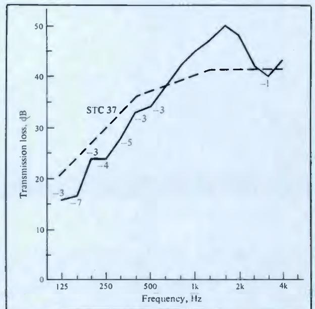
Figure 2. The determination of the STC for the measured values of transmission loss for a partition of ½-inch plasterboard.
