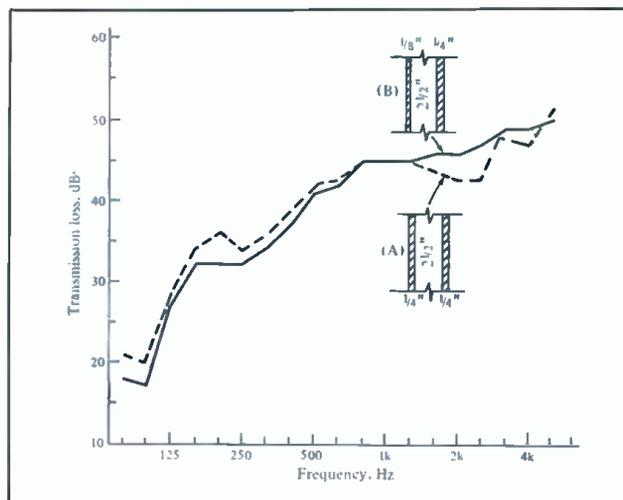
Figure 2. The use of glass of different thickness in double glazed windows serves to minimize the coincidence irregularities by staggering the two coincidence frequencies. Curve A is for a window utilizing two panes of 1/4-inch (6mm) thickness spaced 2 1/2 inches (63mm). Curve B is the same window with one glass reduced to 1/8 inch (3mm). (Adapted, with permission, from Quirt, Ref. 1.)
