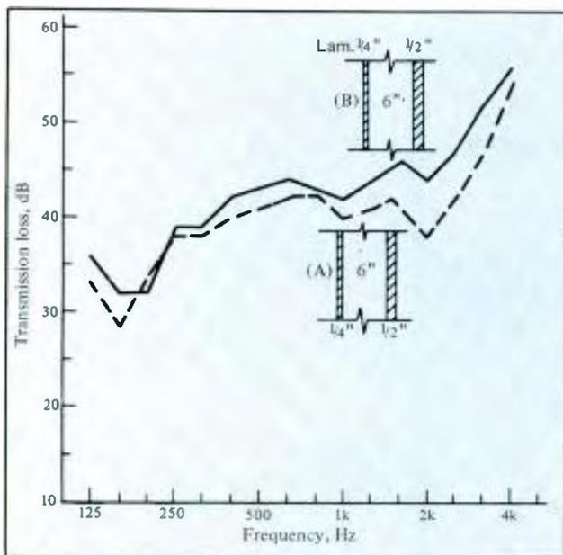
Figure 3. Laminated glass offers less stiffness than comparable solid glass: (A) Normal double glazed window of  $\frac{1}{4}$ -inch and  $\frac{1}{2}$ -inch glass sheets spaced 6 inches; (B) the same window except the  $\frac{1}{4}$ -inch solid sheet has been replaced by two  $\frac{1}{8}$ -inch sheets laminated with 0.045 inch plastic. The window with the laminated sheet shows the greater transmission loss. (Libby Owens Ford, Ref. 3.)
