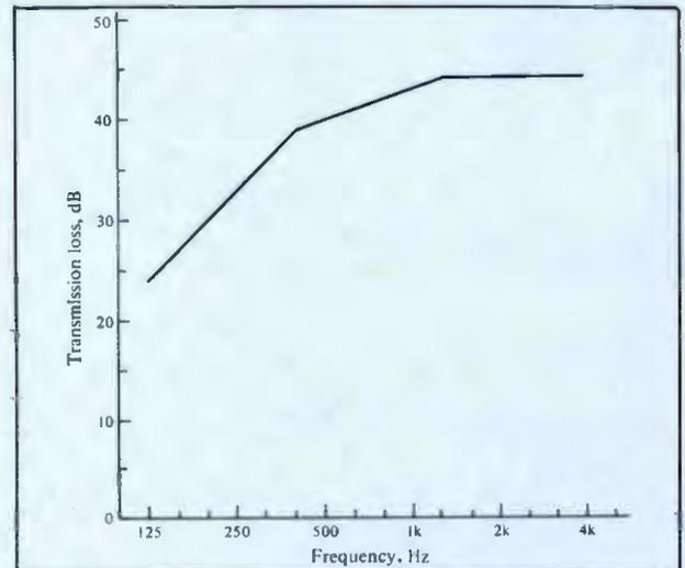
Figure 1. The standard STC contour.
