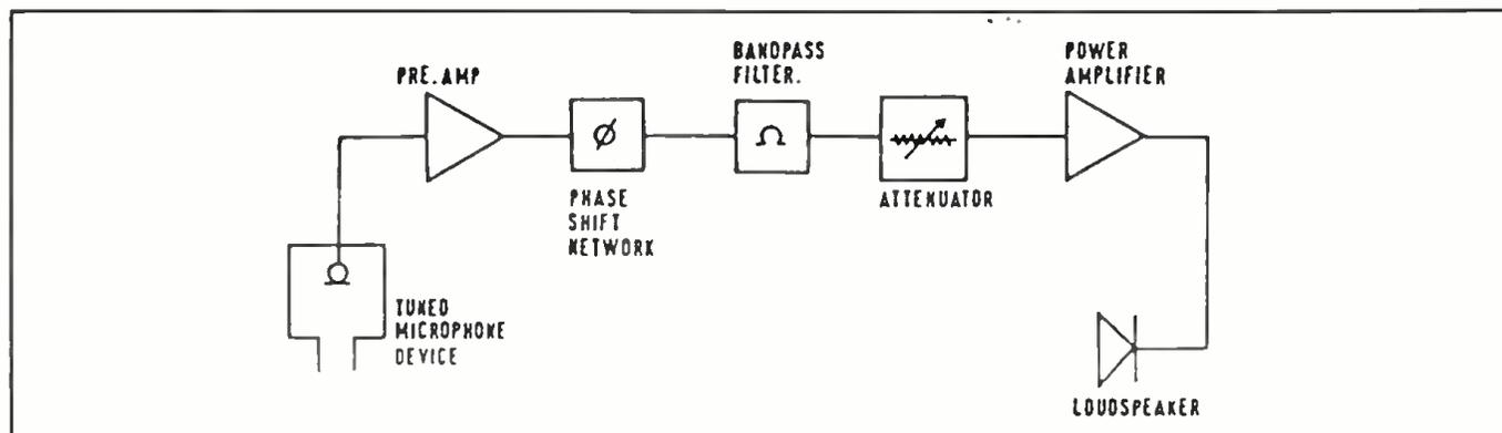
Figure 1. Block diagram of the basic system channel.
