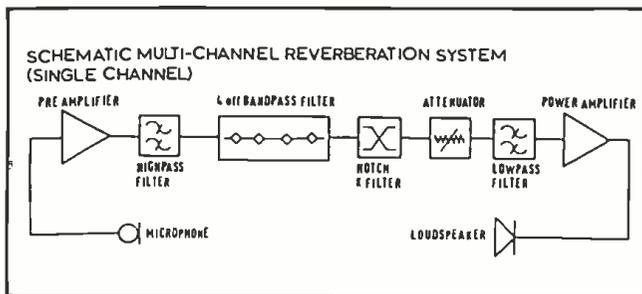
Figure 4. Simplified block diagram of basic reverberation system.
