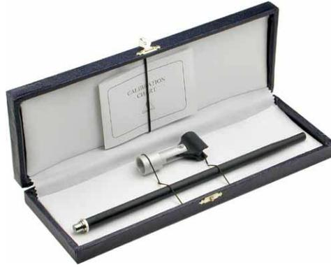
The MIC-01 microphone is an electret measuring microphone that is particularly well suited to be used in conjunction with the other components of the CLIO system. It is furnished with its own stand adaptor and a calibration chart reporting the individually measured sensitivity, all fitted in an elegant case. Its long and thin shape renders it ideal for anechoic measurements. Because its frequency response is very flat over the entire audio band, no particular correction is usually needed.
