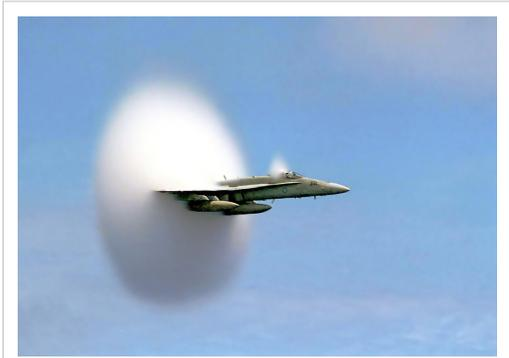
When an aircraft is near the sound barrier, an unusual cloud sometimes forms in its wake. A Prandtl-Glauert Singularity results from a drop in pressure, due to shock wave formation. This pressure change causes a sharp drop in temperature, which in humid conditions leads the water vapor in the air to condense into droplets and form the cloud.
