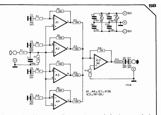
IC operational amplifiers seem to offer an attractively simple means of building audio preamps, but unfortunately ICs generally offer inferior noise performance to the best discrete circuits. However, as quad op-amp ICs are now available at modest cost a novel solution to this problem is possible. If a number of identical amplifiers are fed with the same signal and the outputs are
