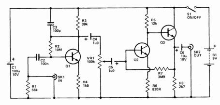
Microphones provide only a minute output signal and cannot be used successfully with many items of equipment unless their output is augmented by a suitable preamplifier. For example, few stereo Hi-Fi amplifiers have an input that is an acceptable match for a microphone (a magnetic pickup input is unsuitable as it has RIAA equalisation with consequent bass boost and treble cut). Many simple mekers have only high level inputs and require separate preamplifiers for use with low level sources.
