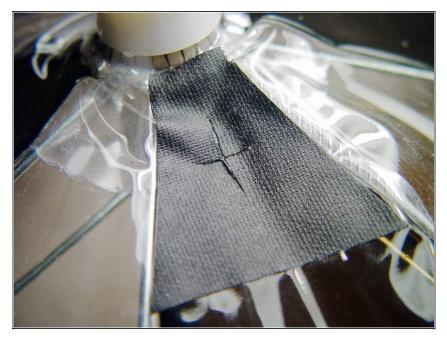
Cover 1 gore of the umbrella near the center with a trapezoidal piece of the gaffer's tape. Cut a small Xshaped incision through the tape and umbrella; this will be the reinforced hole that the microphone wire will pass through.
