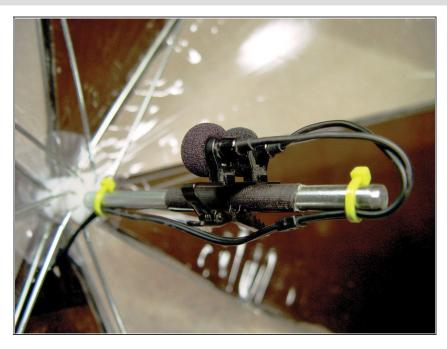
Clip the mic to the shaft and thread the cable through the X hole.
