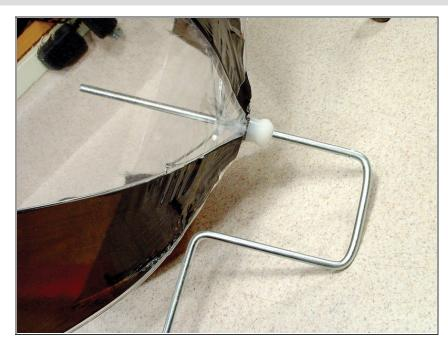
Remove the paint roller's plastic caps and wire frame. Push the shaft through the hole in the top of the umbrella, so that it protrudes 6" underneath. Leave ½" of clearance between the outer surface of the umbrella and the bend of the handle.
