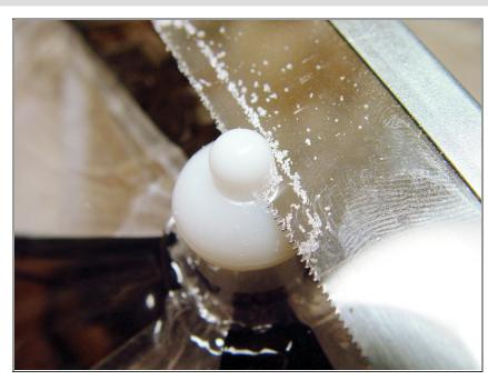
Slice the top of the plastic knob off the top of the umbrella, and clean up the hole with a knife or reamer.
