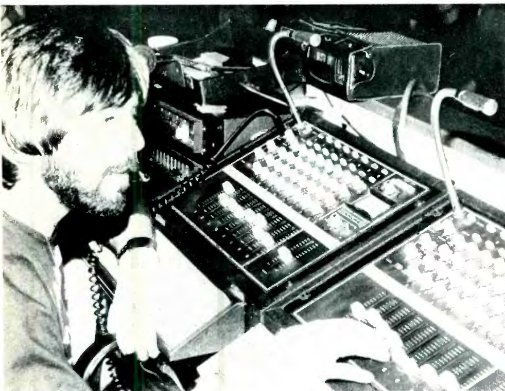
Romano at work with the Shure M67 Mixer and the M610 Feedback Controller to get a proper acoustic balance in the auditorium.
