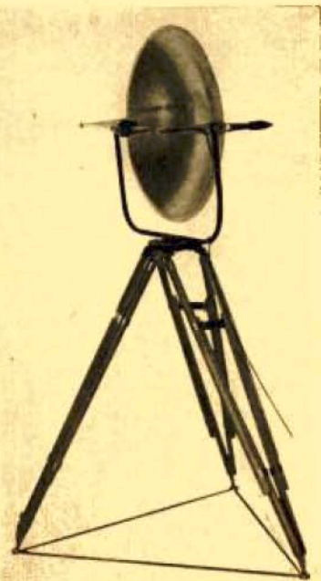
Fig. 2. The complete parabolic microphone unit mounted on a tripod.
