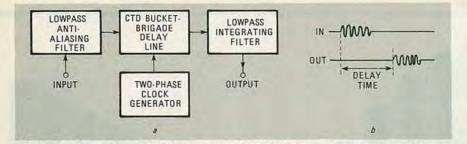
FIG. 1—AN ANALOG DELAY LINE is composed of a bucket-brigade delay line, input and output lowpass filters, and a two-phase clock (a). The circuit produces a time-delayed replica of the input signal (b).
