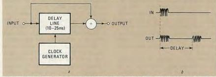
FIG. 5-THE DOUBLE-TRACKING CIRCUIT, or micro chorus, mixes the input signal with a delayed replica of the input signal (a). Input and output waveforms are shown in b.
