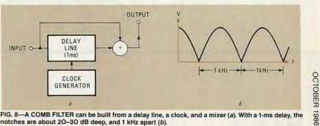
FIG. 8—A COMB FILTER can be built from a delay line, a clock, and a mixer (a). With a 1-ms delay, the notches are about 20-30 dB deep, and 1 kHz apart (b).
