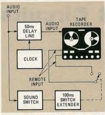
FIG. 14—A SOUND-ACTIVATED RECORDER that does not miss sound input can be built using an analog delay line.
