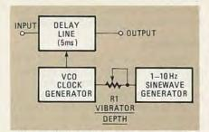
FIG. 4-THE VIBRATO CIRCUIT frequency modulates the input signal with a low-frequency oscillator.
