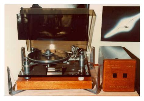
This is my turntable (Oracle Delphi, SAEC 407/23 tonearm, Dynavector Karat 23R "Ruby" pickup) mounted on an "antisismic" support (a wood tablet filled with concrete and suspended). On the right side, the moving-coil preamp.
