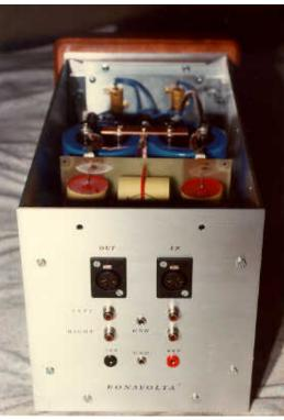
The power supply are two batteries in // with super-caps (1Farad), electrolytic capacitors (560'000uF) and several stages of various types and sizes of smaller caps until the high-speed polypropylene (Leclanché with extremely high slew-rate).
