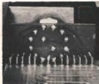
Above: rear view of the selector switch PCB. You may have to shorten two of the PC pins to stop them fouling the switch terminals.
