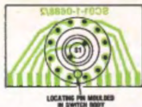
Fig. 5: the selector switch should be mounted on its PCB with the locating pin towards the bottom. Check the PCB pattern carefully to ensure that none of the input pads are shorted together.
