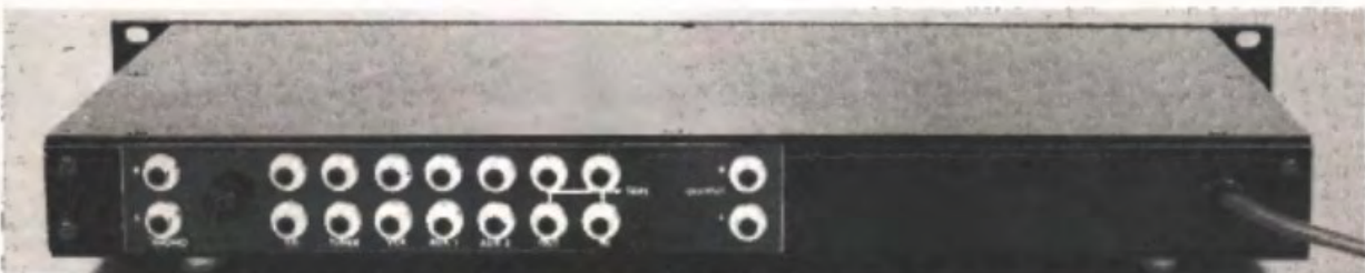
The rear panel carries the RCA input and output sockets, an earthing terminal and the mains cord grommet.
