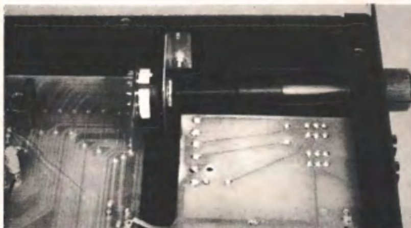
The switch assembly is soldered at right angles to the phono preamplifier PCB and supported by an L-shaped bracket secured to the side rail. The switch shaft is lengthened using an extension shaft and coupler.
