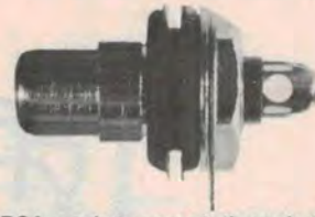
The RCA sockets mount through the hole of rubber grommets fixed to the rear panel, electrically isolating them from the panel.
