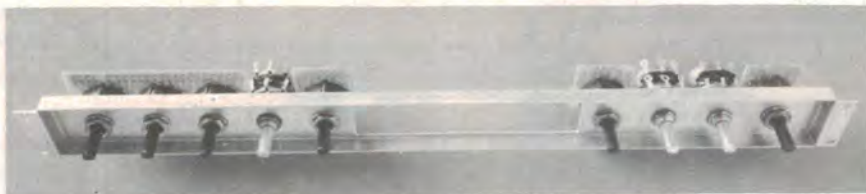
Switch assemblies and potentiometers, with their shafts cut to length to suit the knobs used, mounted to the sub-panel.
