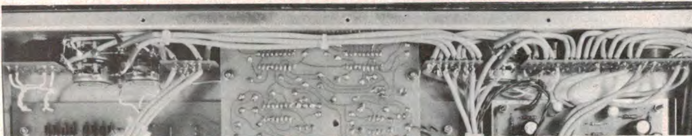
View of the rear of the sub-panel assembly, which holds all the switches and potentiometers. Wiring to the switches is from small pc boards mounted on the rear of each switch. This greatly simplifies the
