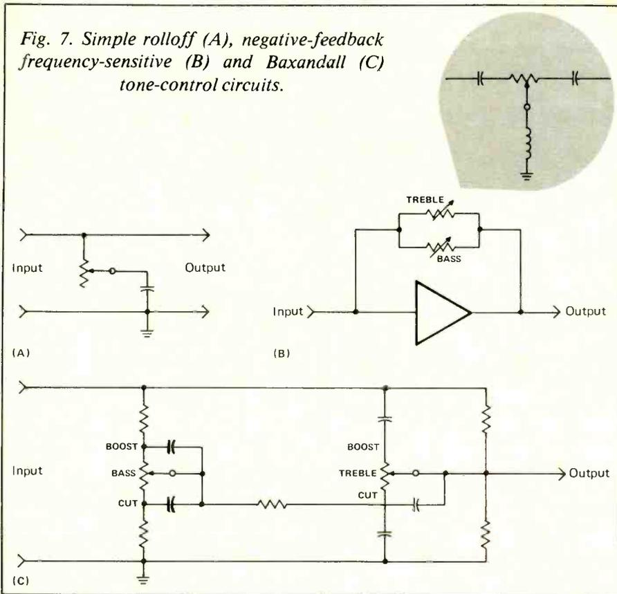
shown in Figure 7B. In this version, a pair of frequency-sensitive RC or RLC networks is placed in the negative-feedback circuit of the amplifier. These circuits selectively amplify different bands of frequencies. An example of the RLC version is shown in the inset in Fig. 7B.
