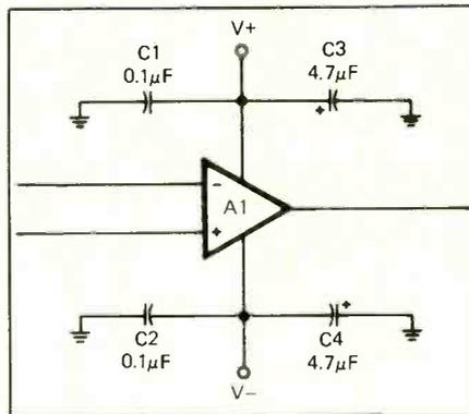
Fig. 1. To assure stable operation, it may be necessary to bypass each power-supply line with two capacitors to handle entire audio range.
