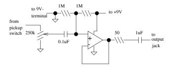
The opamp is a LT1012 micro power opamp, could be other low noise low power op amp. Use a stereo jack on the guitar to turn power on when a cable is plugged in. The circuit produces no noticeable noise or distortion and a 9 volt battery lasts a couple of years. This is intended to buffer the guitar pickups and controls from the cable capacitance. It is possible to add gain to this circuit by modifying the
