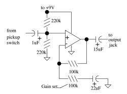
A preamp from a TL071 op amp. The gain set resistor lets you customize the gain. As shown, it is 2. Lowering the Gain Set resistor lets you raise the gain. You get distortion at high gains.
