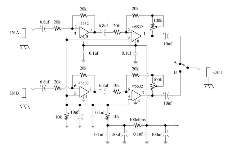
This low noise preamp & a/b box was originally designed for switching between different harmonica mics.
