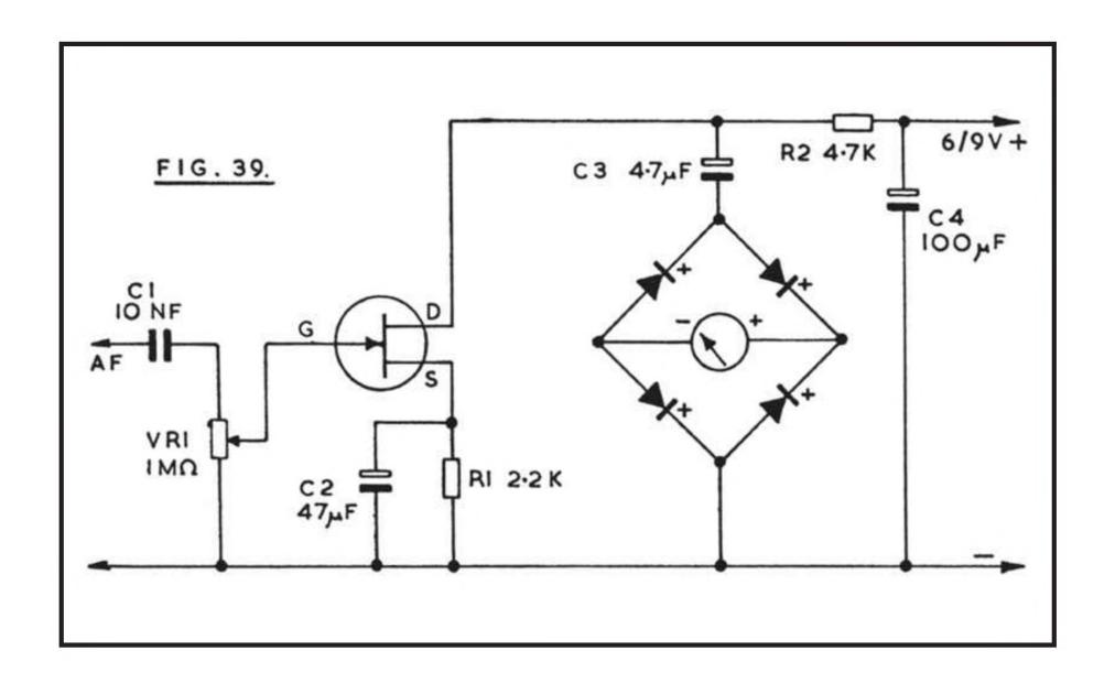
Audio power from the drain develops a voltage across R2, and is coupled to the full-wave rectifiers by C3. Current from these flows through the meter, so that a reading is obtained which depends on the strength of the audio signal.
