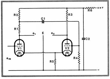
to the gain of V2. It is usual, therefore, to make the tapping point variable and to adjust it under working conditions. When  $R_3=R_1+R_2$ , the valves are similar, and  $e_1=e_2$ , the alternating components of the anode currents through R5, are equal and opposite. No by-pass condenser is consequently needed to prevent negative feedback.
