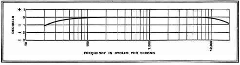
Fig. 9.—The frequency-response, including the output transformer, shows a drop of about I db. at 20 c/s and 20,000 c/s.
