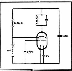
The circuit diagram and valve characteristic curve enclosed with Mr. Lea's letter. Do they disclose the reason for the failure to oscillate? ting anything to oscillate. I have checked over all the connections many times and tried tuned circuits that I know should oscillate easily with the slope of this valve. Having heard that you are good at solving these little mysteries, I am writing in the hope that you will do me this favour.
