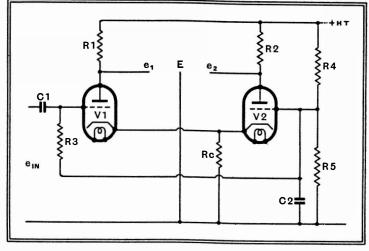
Fig. 5.-A new phase-splitting circuit is shown here. V2 derives its input from the cathode circuit of VI. There is some negative feed-back on VI.
