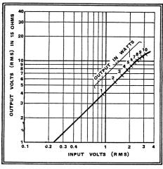
Fig. 8.—The input-output curve of the amplifier is linear up to 7 watts or slightly more.
