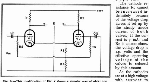
Fig. 6.—This modification of Fig. 5 shows a simpler way of obtaining grid bias by the voltage drop across R3.
