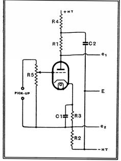
Fig. I. – This phase splitter is simple and gives high gain, but neither input terminal can be earthed.
