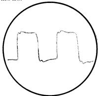
Fig. 3. Oscillogram of 5000-cycle square wave after passing through this amplifier. This indicates good transient response.
