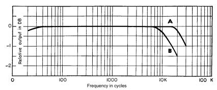
Fidelity response curve of high-quality amplifier. In (A), output power is one watt.
