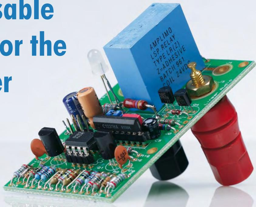
A good protection system for an audio amplifier has two important tasks: speaker protection and amplifier overload protection. Speaker protection concerns a possible excessive DC voltage at the amp output due to either excessive ultra-low frequency signals, or from a circuit failure inside the amp. By the way, you can also get excessive DC output if you have a DC coupled power amp and your preamp gives out DC. If you go on tour with your amp, it would be wise to insert
