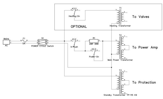
Optional part of the schematic is relevant in case you've got valves in the circuit.
