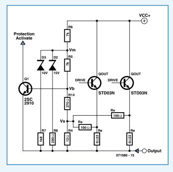
Figure 2. SOA protection circuit.
