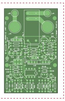
Figure 4. Component placement of the double-sided PCB for the o/p board.
