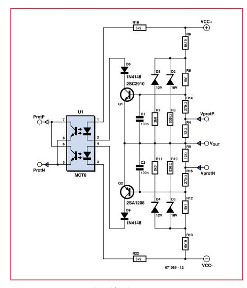
Figure 2. Safe Area Protection system.
