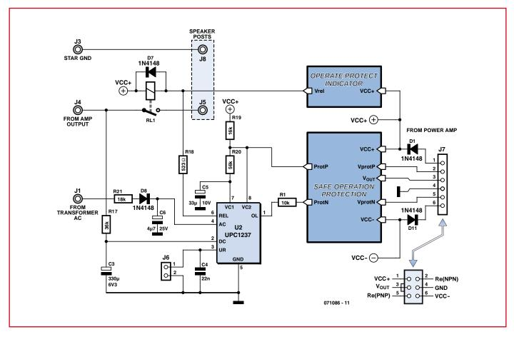
Figure 1. Overall protection system.
