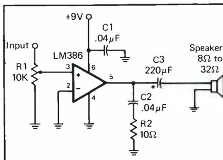
Fig. 1. Basic LM386 amplifier circuit. Place *C1* as close as possible to the LM386 integrated circuit.
