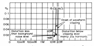
Fig. 6. Power output/distortion characteristics. The  $8-\Omega$  load characteristic was measured using the modified output-stage components.
