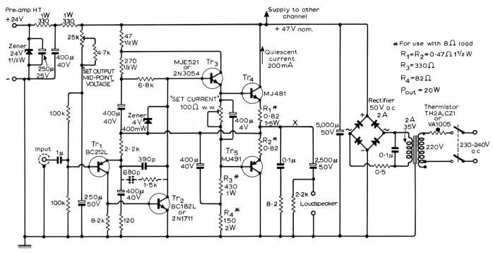
Fig. 3. Power amplifier circuit. The dotted components (680 pF, 1.5k $\Omega$ ) can be added if electrostatic speakers are used.
