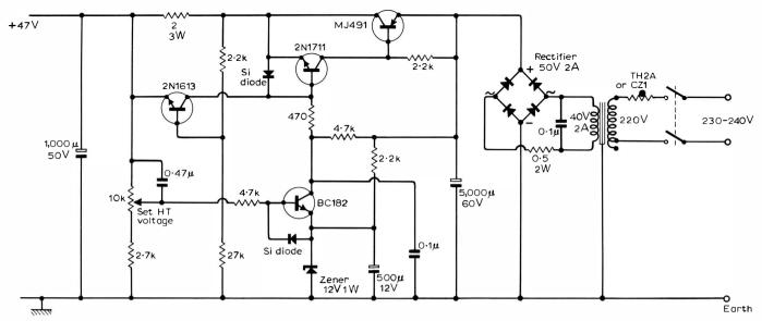
Fig. 10. Stabilized power supply with re-entrant short-circuit protection (12-49V).
