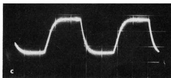
Fig. 8. Square-wave performance into  $15\Omega$  in parallel with 0–0.1 $\mu$ F. (Scale 2V/cm) (a) 1kHz, (b) 10kHz, (c) 50kHz.
