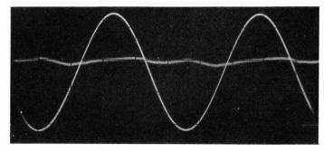
Fig. 9. 14-W 1-kHz sinewave into 15- $\Omega$  resistive load. Distortion 0.018% on scale 35mV/cm. Fundamental on scale 10V/cm.
