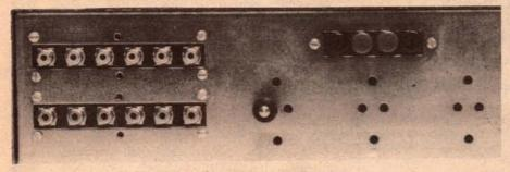
At the top of the page is a plan view looking into our new "Twin Ten" Playmaster amplifier. The uncrowded layout should make for easy construction. The partial back view shows the input sockets (left), the loudspeaker terminals (right) and an earth terminal for possible connection to the phono player deck. If the amplifier is built on the twin-25, Twin-40 metalwork, the output transistor mounting holes will remain unused.
