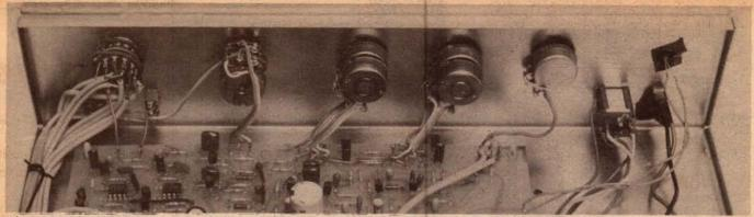
Above: Looking behind the front panel at the controls and associated wiring. On the left is the selector switch and, almost hidden below it, the stereo/mono and tape monitor switches. The sequence of the other controls can be deduced by comparison with the front view on the title page. Note the use of lacing and of ribbon leads to the controls, in the interest of neatness.
