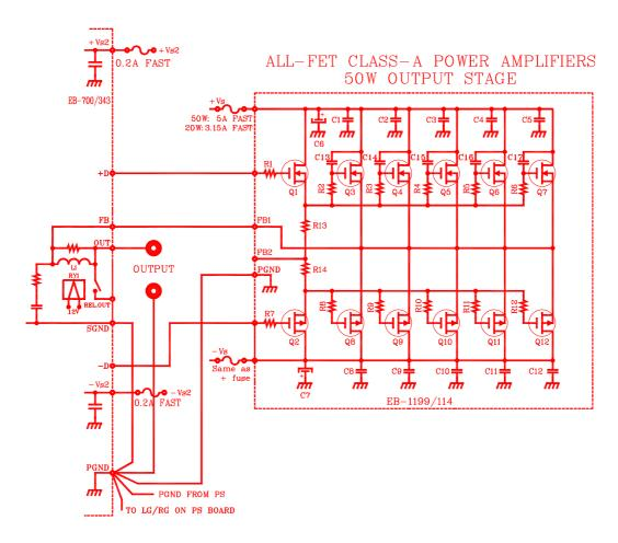
Fig. 3. The EB-1199/114 ALL-FET Class-A output stage.
