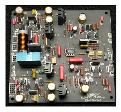
Fig: 5. The RIBBON driver on Teflon PCB, with Caddock upgrade.
