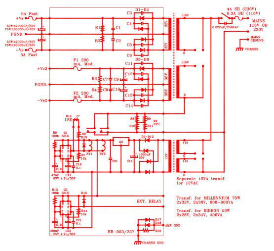
POWER SUPPLY FOR ALL-FET 50/75W CLASS-A MONO BLOCKS EB-903/237/PS75W237
