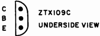
Fig. 5—Identification of leads of ZTX-109C. NOTE: THIS IS THE VIEW FROM UNDERNEATH.
