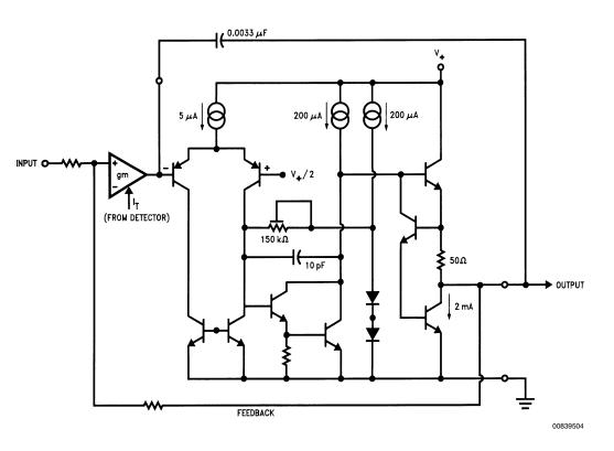
FIGURE 4. The OP AMP Output Stage of the LM1894
