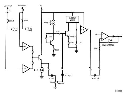
FIGURE 5. Control Path Amplifiers and Filters
