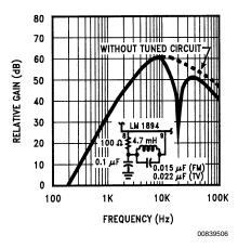
**FIGURE 6. Control Path Frequency Response**
