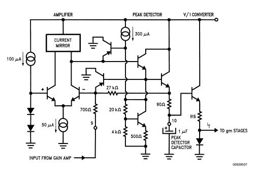
FIGURE 7. Peak Detector and Voltage to Current Converter
