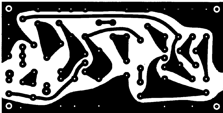
Fig. 2. The actual size foil pattern and component layout. Observe the polarities carefully during assembly.
